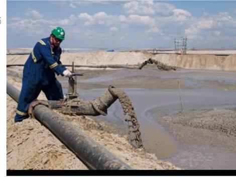
Suncor pumps a slurry of mature fine tailings and polymer flocculant over a gently tilted slope for drying. The TRO process works only during seasons without freezing weather.
