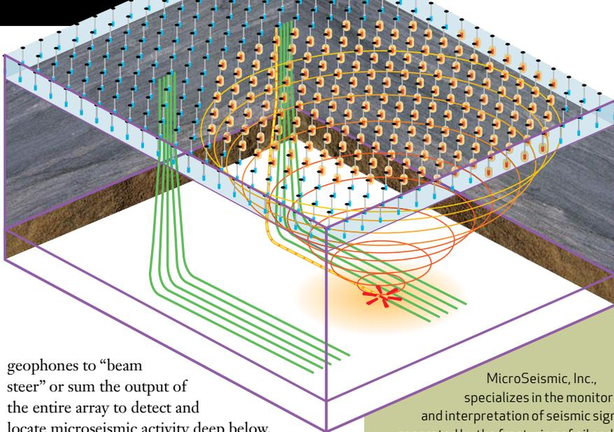
geophones to "beam steer" or sum the output of the entire array to detect and locate microseismic activity deep below.
