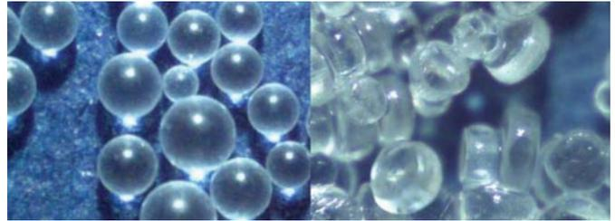
weight proppant, working with a third party. With its specific gravity of 1.05, compared to sand with a specific gravity of 2.65, the LWP travels more easily and about three times farther than a conventional proppant like sand.
