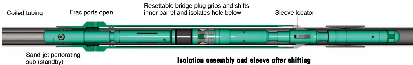
Plug & perf and ball-sleeves and packers are basically brute-force techniques, with fluids and fracs bullheaded down the casing and into the formation, with no feedback about formation response at the frac zone, no recourse in the event of a screenout, and no way to conserve water and chemicals. Also, both methods can require extensive post-stimulation work to drill out plugs or ball seats.
